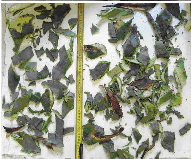
Figure 1 (top) Prototype being tested on an Agave plant. Figure 2. Residue size after chopping.
