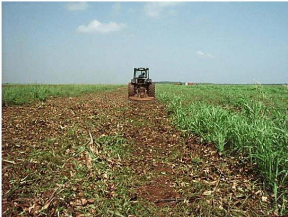
Figure 2. Chopping residue in a weed-infested field with the CH-60 mower.
